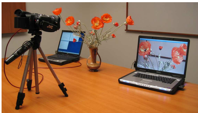
Figure 1. HD transmission over a wireless, ad-hoc link (802.11a) between two laptops in the laboratory.
