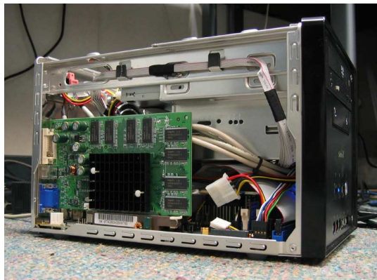
Figure 4: MPEG-2 decoding is achieved with a Nvidia FX 5200 based graphics card. The Linux supplied drivers accelerate the iDCT and motion compensation steps required for MPEG-2 decoding.
