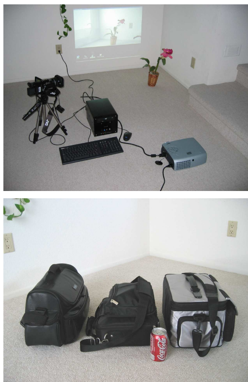
Figure 3: High definition video streaming equipment. Top: A Shuttle XPC computer complemented with a JVC JY-HD10U camera and a DLP projector are the minimally required equipment at each user location. (In the picture, the local video of the camera is displayed.) Bottom: The setup is quite portable – from left to right: the camera, the projector, and the computer bag.
